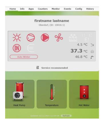
This page shows the basic web application for controlling the heat pump. It is very similar to the end user application and allows quick basic settings such as:
